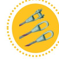
The individual wires of the strands are opened up to form a broom. This broom is inserted into the socket. Molten Zinc is poured into the broom to lock in the joint to form a Spelter lock for Spelter sockets. Alternatively, Wire Locking Resin may also be used to accomplish the lock.
