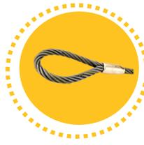
A mechanically spliced wire rope sling is fabricated using an Aluminium, Copper or Steel Ferrule to securely lock in place the splice junction. The difference here is that the Ferrule is swaged into place using a die based hydraulic swaging press, exerting a staggering 3000 tons of force.
